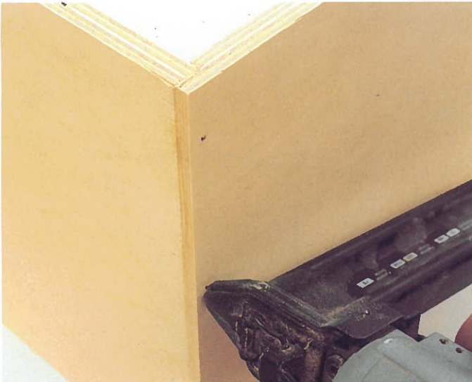
[13] Cut the drawer boards using \frac{1}{8} "-thick Baltic birch plywood. Glue and nail the sides to the front board and backboard.
