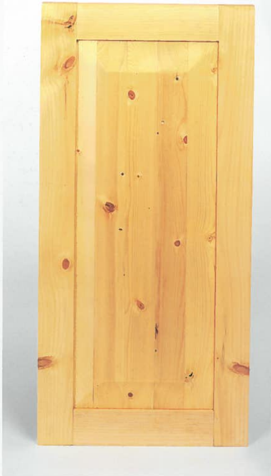
Here's a typical raised panel door like the one you'll build in this demonstration.
