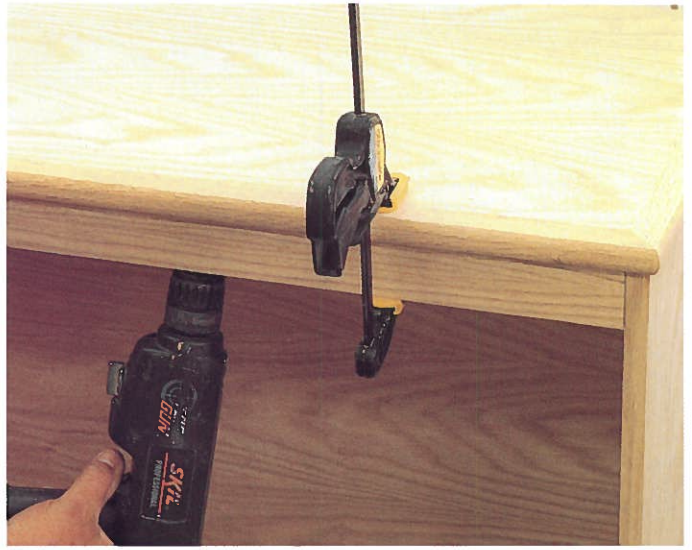
[12] Clamp the top in place so it's flush with the backboard and equally overhanging on each side. Use \frac{1}{8} " screws through the brackets into the underside of the top.
