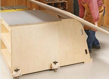
▲ The curved cradles carry the weight of a sheet of plywood to make it easy to tilt it up onto the table. Then just slide it over to the table saw to make a cut.
