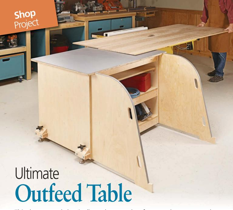
This shop upgrade has it all — a large worksurface, ample storage, and a unique sheet goods lifting system. Plus, it's easy to roll-around the shop.
